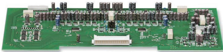
■ AAVA volume control assembly minimizes noise
